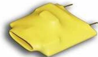
Amplifier manufacturers and aftermarket manufacturers of replacement amplifier modules are offering plug in surge protectors to protect amplifiers. The units consist of a plug in crowbar surge protector. A crowbar device consists of 2 SCRS and a diode to trigger the device. The device senses an overvoltage and shunts it to ground, much like a Sidactor. These units are offered by the amplifier manufactures as a solution to damage to the amplifier circuitry caused by surges.
